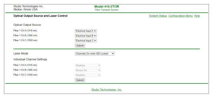
Model 410-3T/3R SDI-Over-Fiber Transport System example Optical Output Source and Laser Control menu page (typical for all Model 410 versions)
