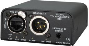
The STcontroller software application is used to select the unit's operating parameters. The talk pushbutton switch can be configured for optimal operation. Two "push-in/push-out" ("pop-out") rotary controls make it easy to set and maintain the desired headphone output level. The Model 373A's compact enclosure is made from an aluminum alloy which offers both light weight and ruggedness. A stainless steel belt clip, located on the back of the unit, allows direct attachment to a user's clothing.
